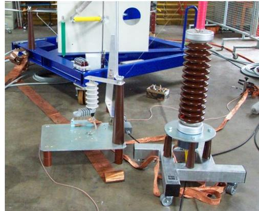
Impulse current testing arrangement for MV arresters
