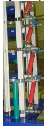
Each resistor value has a specific colour for easy identification. These resistors have a plug-in connection for quick and easy reconfiguration. The basic system includes a set of resistors for lightning impulse voltages according to IEC 60060-1.
