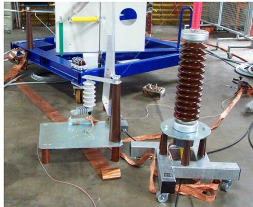
Impulse current testing arrangement for MV arresters
