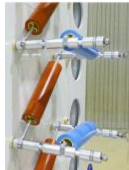
They are the wave shaping elements and wire-wound for high stability and linearity and are wound on tubes and protected by shrink wrap or compound moulding.
