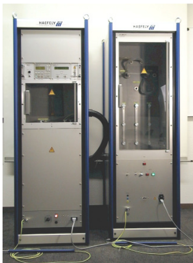
PSURGE 30.2 generator rack (left) with FPSURGE 3010 coupling network (right)
