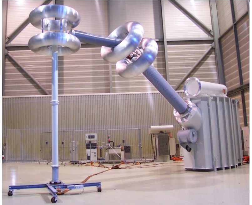
700kV Transformer with Oil to air bushing
