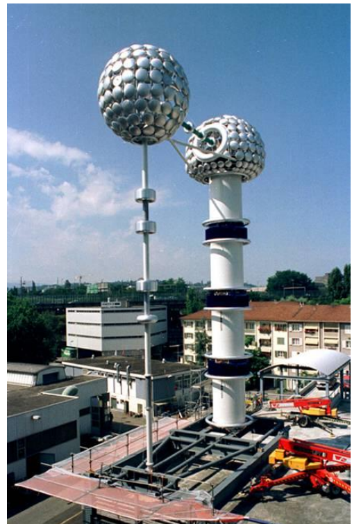
Example of 1'500 kV, 1.2 A cascade made of 4 transformers
